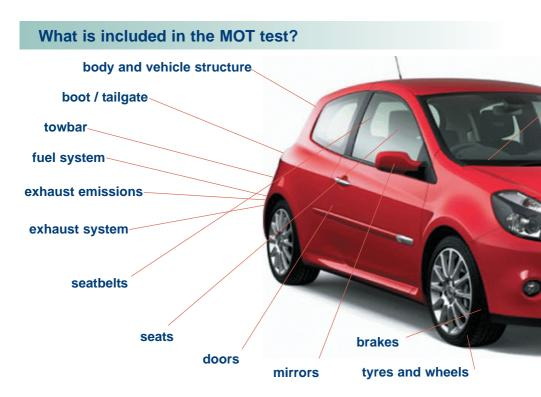
**Body & vehicle structure:** Free from excessive corrosion or damage in specific areas, no sharp edges likely to cause injury, towbars for security and condition
